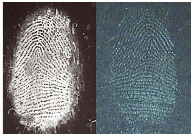
FIG. 7—Latent fingerprints deposited onto glass surfaces following 52 weeks of storage at 20°C and developed using cyanoacrylate fuming (SUPERfume ® ) (left) and developed using aluminum powder dusting (right).
